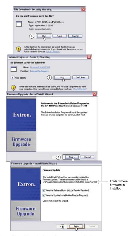
Figure 5-10 — Downloading firmware upgrade files
